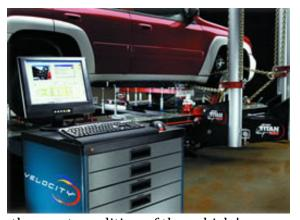
Fast and easy set-up with full-color, one-page reports on the exact condition of the vehicle's frame before, during and after repairs have been made for indisputable evidence of damage severity and quality repairs.
