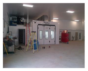
built with two inch by two inch square tube frames for heavy duty service, and have a heavy lip for air seal. One 36" × 84" personal access door is standard.
